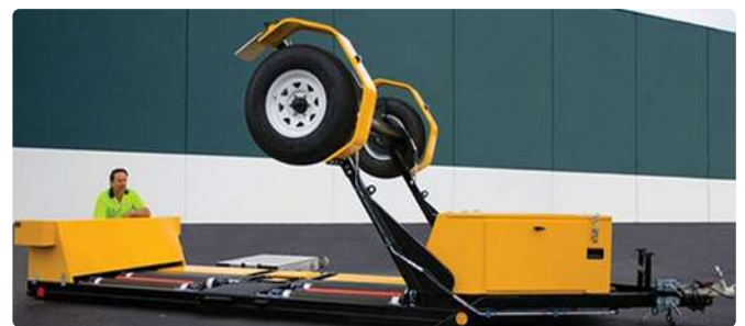
A portable PBBT unit used for deployment outside of a fixed maintenance location. Unit pictured is VIS-Check portable unit.
